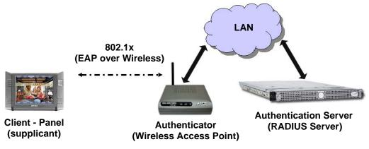
FIG. 86 EAP security method in process
